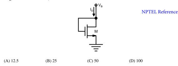
Q.35 The ac schematic of an NMOS common-source stage is shown in the figure below, where part of the biasing circuits has been omitted for simplicity. For the *n*-channel MOSFET M, the transconductance  $g_m = 1 \text{ mA/V}$ , and body effect and channel length modulation effect are to be neglected. The lower cutoff frequency in Hz of the circuit is approximately at
